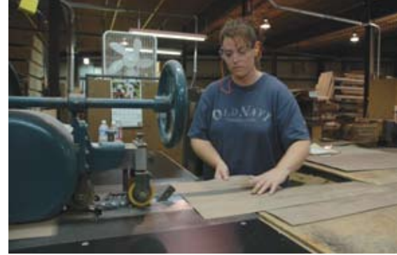
Veneer is spliced from faces and backs to be used in plywood.
