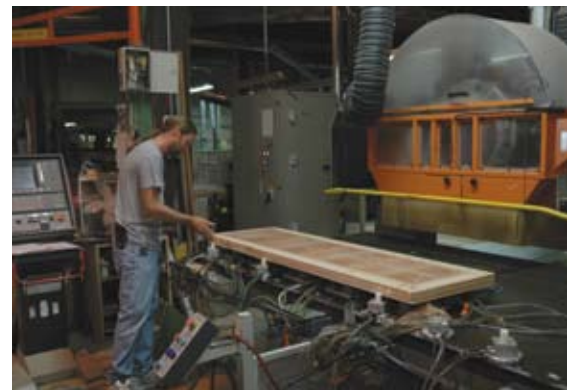
An employee sets up the CMS router to machine a plywood top containing a special sketch face.
