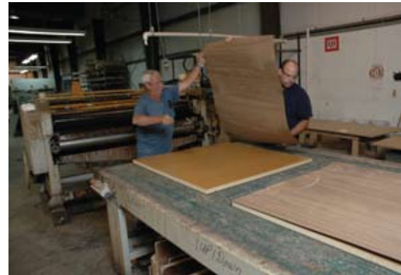
Plywood operators show the lamination of faces, backs and cores.
